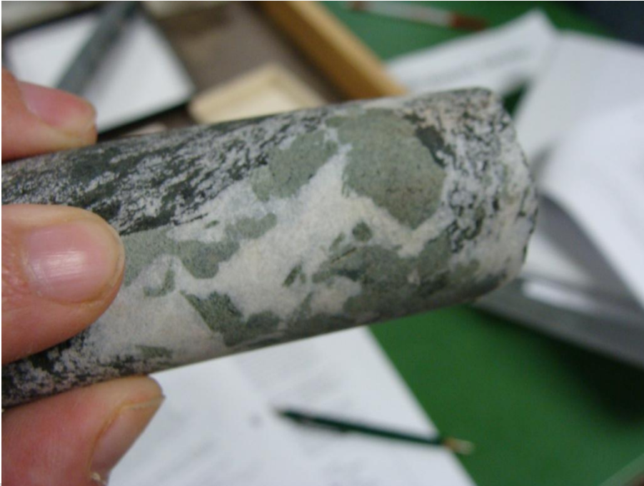
78001-93.6: Multiple generations of actinolite/albite cutting biotite shist
