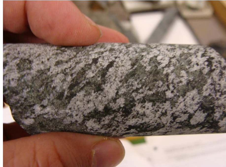
78601-56.6: Multiple generations of actinolite/albite cutting biotite shist
